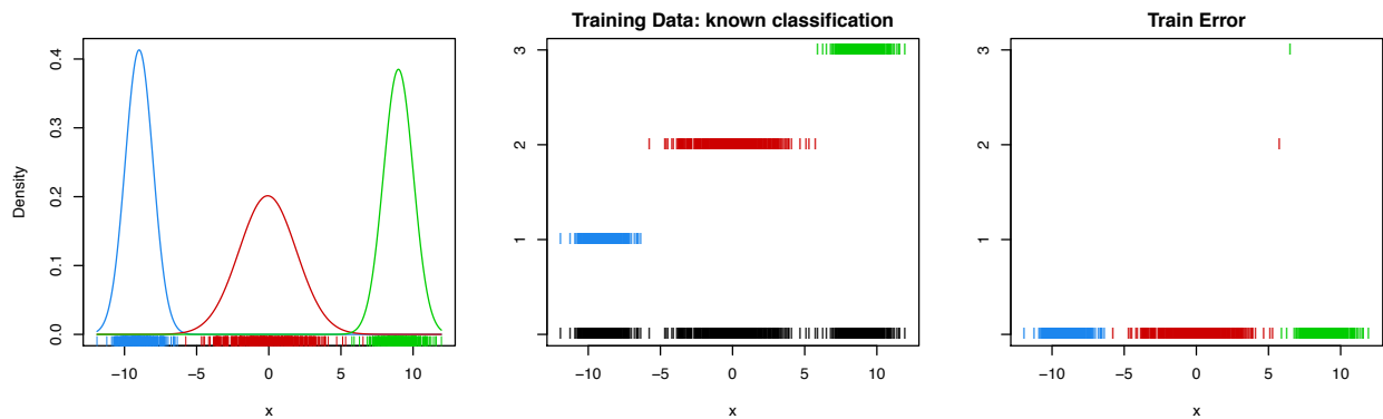
Figure 18: LEFT: Densities for the univariate simulation data. There are two components with variance 1 centered at -9 and 9, respectively, and one component with variance 4 centered at 0. CENTER: Training step classification. RIGHT: Misclassified training observations.
