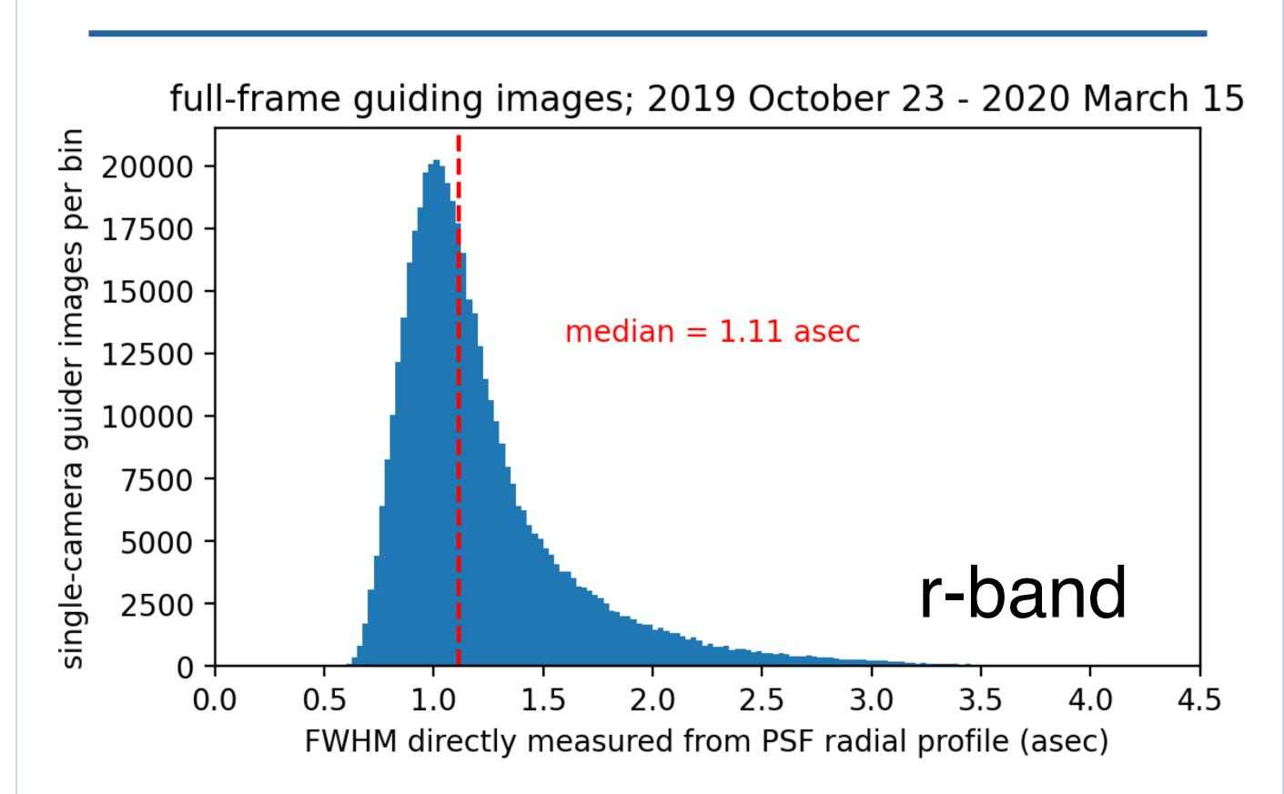
FWHM distribution for ~500,000 full-frame DESI guider images on 92 observing nights. The median FWHM of 1.11" is very similar to the pre-DESI R-band median<sup>6</sup> FWHM of 1.17".
