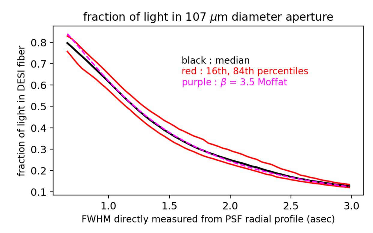
Fraction of light entering a 107 micron diameter DESI fiber as a function of FWHM. The measured trend (black) is almost identical to that expected for a  $\beta$  = 3.5 Moffat profile (purple).
