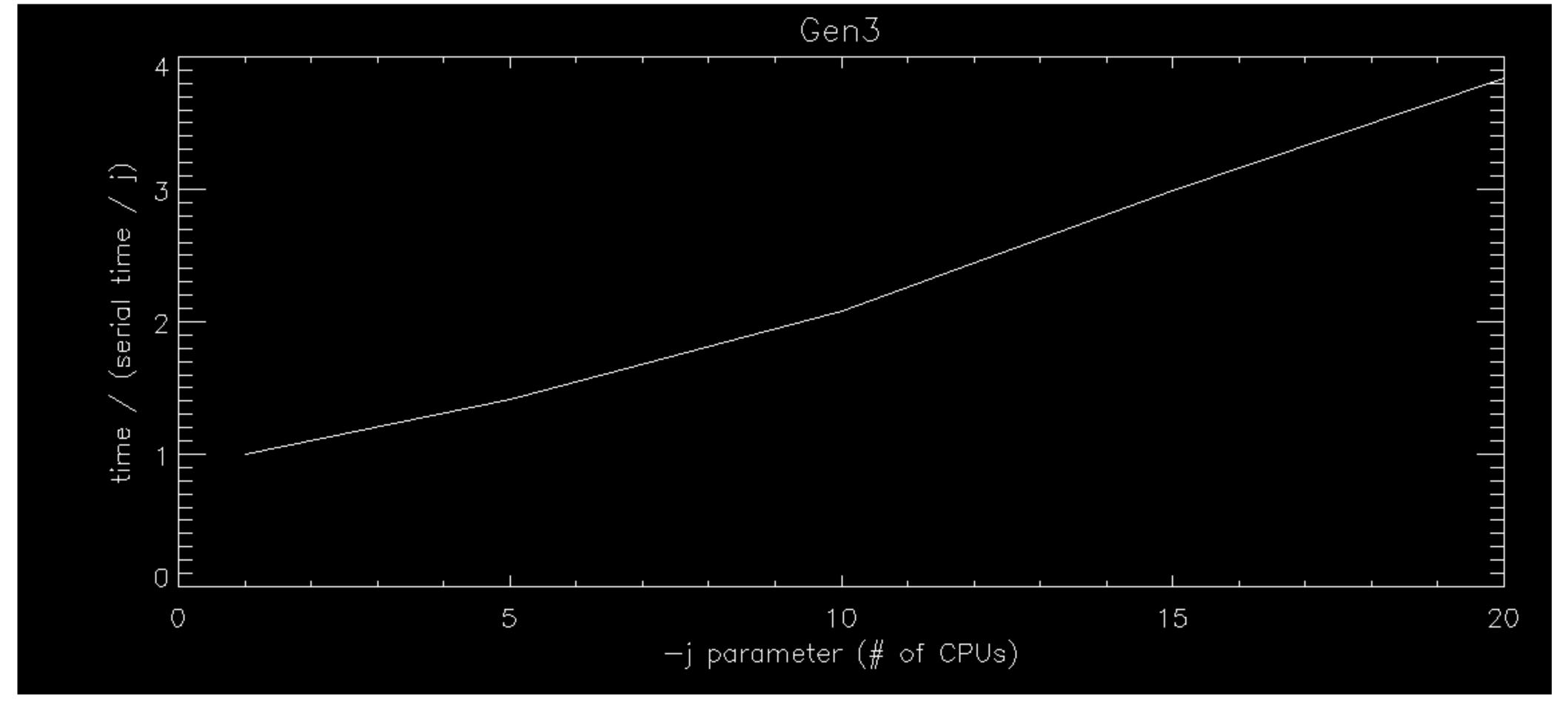
scaling relative to serial is  $\sim$ 2.5x worse at j = 20 for Gen3 relative to Gen2
