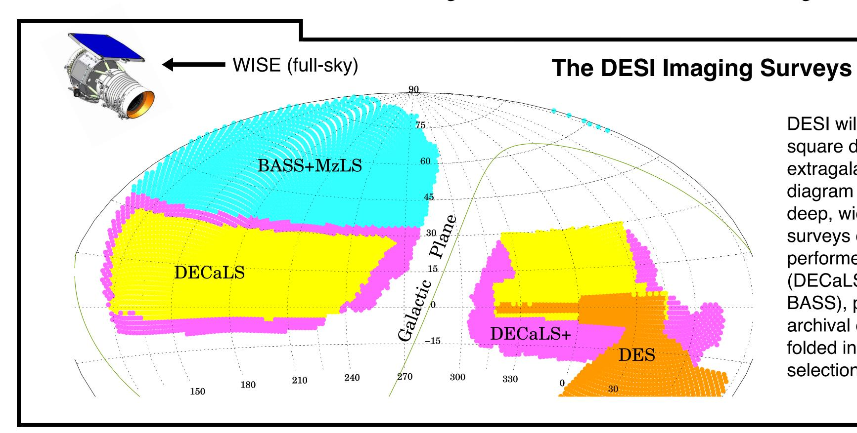
DESI will observe ~14,000 square degrees of extragalactic sky. The diagram at left illustrates the deep, wide-field imaging surveys currently being performed to enable DESI (DECaLS, DECaLS+, MzLS, BASS), plus additional archival data sets being folded in to DESI target selection (WISE, DES).
