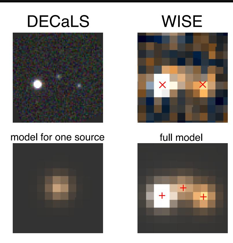
DESI imaging reductions employ an inference-based approach to model sources across a wide range of wavelengths. The top left plot shows a DECaLS g+r+z composite. Because the DECaLS data have much higher spatial resolution than the mid-infrared WISE images, a "forced photometry" technique is used to extract infrared fluxes by fitting a model with source centroids and morphologies fixed to those measured in the optical.
