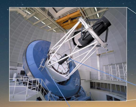
DESI is a highly multiplexed optical multi-fiber instrument installed at the 4-meter Mayall telescope at Kitt Peak, AZ.
