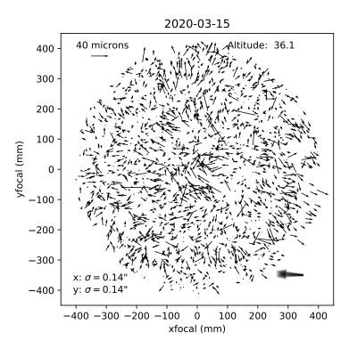
Figure 3: Fiber positioning errors for a sequence of exposures taken at a zenith distance of 54°. The RMS of 13  $\mu m$  is very close to the high-altitude performance of 11  $\mu m$ . The larger salt-and-pepper noise suggests that the analysis is limited by the larger statistical uncertainty on this field as compared with the high altitude field, owing to the lower stellar densities and therefore fainter typical stars present on this field.
