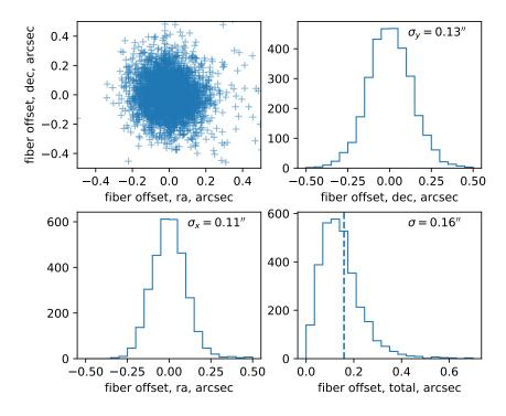
Figure 1: Fiber positioning errors for a sequence of exposures with dithered fiber positions taken 9° from zenith. The four panels show the distribution of fiber positioner errors in 2D, and in y, x, and overall offset individually. The lower right panel shows our final result of 0.16'' overall positioning RMS.
