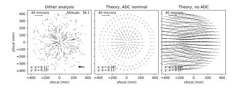
Figure 5: Difference in locations of light centroids in the focal plane at different wavelengths, as in Figure 4. This field, however, is at a zenith distance of  $54^{\circ}$ . Even at this high airmass, the observed centroid differences (left) are consistent with the predictions from ray tracing (center). Absent an ADC, a large, > 1'' constant offset between the different bands would be present (right).
