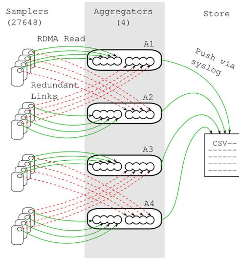
Figure 5. LDMS configuration on *Blue Waters*. Note that this includes redundant connections to each sampler `ldmsd` for fast fail-over capability
