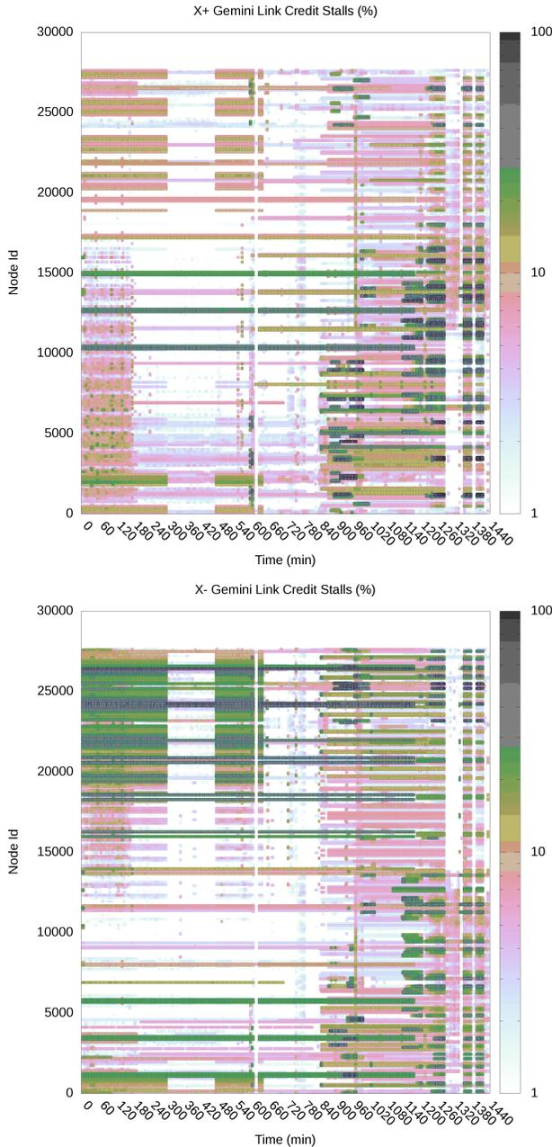
Figure 11. Link aggregated percent of time spent in credit stalls in X+ (top) and X- (bottom).
