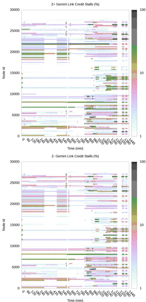
Figure 13. Link aggregated percent of time spent in credit stalls in Z+ (top) and Z- (bottom).
