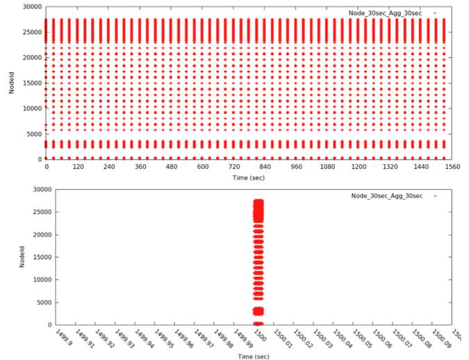
Figure 4. Synchronized sampling and collection over 10,000 *Blue Waters* compute nodes. Y-axis is node number. The top plot shows 30 second collection intervals over a 1500 second time window. The bottom plot zooms in on a particular collection interval to show the tight grouping.
