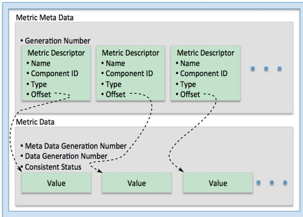
Figure 2. Diagram of LDMS Metric Set Memory.
