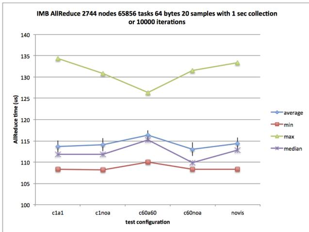
Figure 8. Intel MPI Benchmark results at small scale.
