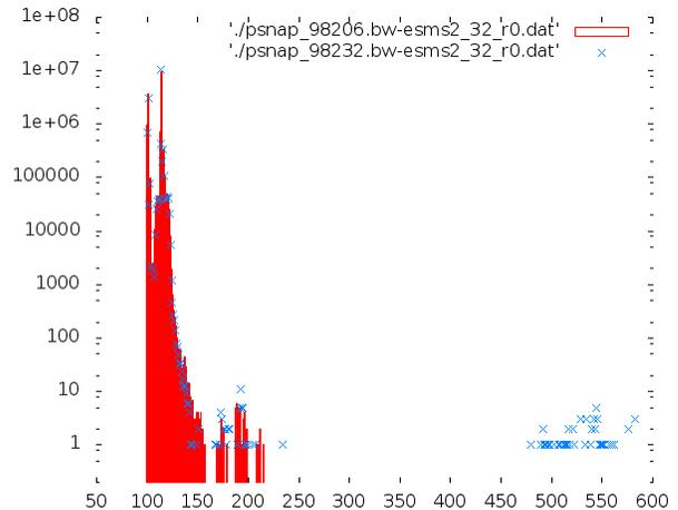
Figure 7. PSNAP results: Histogram of occurrences vs. loop time (us) with 1 second sampling data (X) compared to none (red boxes).
